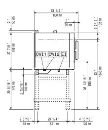
Cold Water inlet 1 (cleaning) CWII Electrical inlet (power) Cold Water Inlet 2 (steam CWI2 generator)
